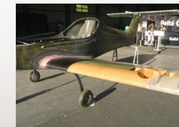
CORE NL10: 332 kg/m<sup>3</sup>, bending strength = 401 Mpa
