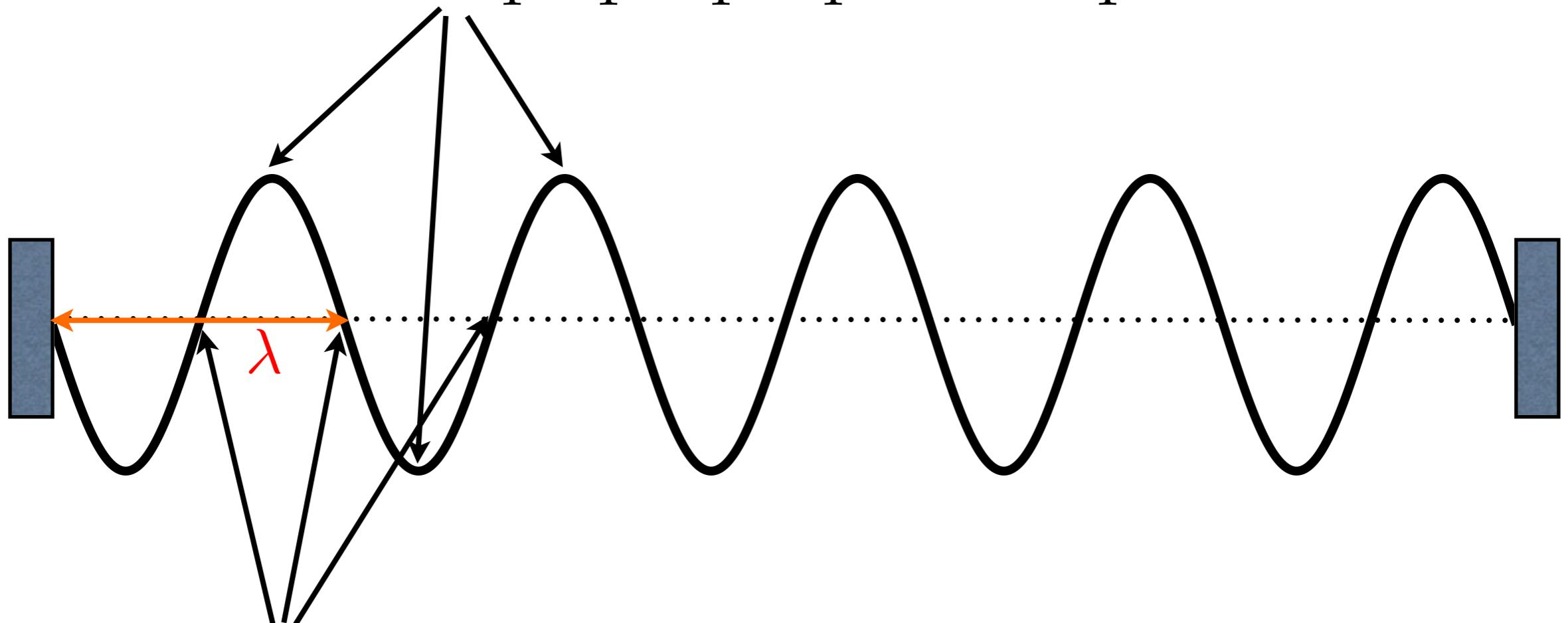
Nodos:  $\frac{\lambda}{2}, \lambda, \frac{3\lambda}{2}, 2\lambda, \dots = \frac{n\lambda}{2}$   $n = 0, 1, 2, 3, \dots$
