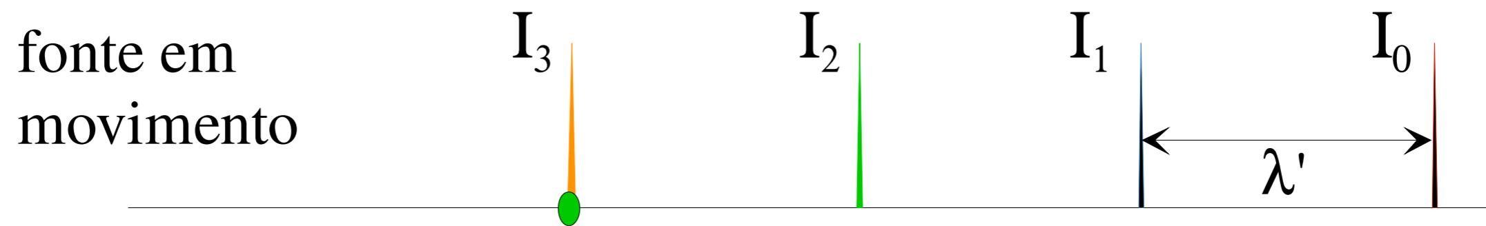
$$\lambda' = \lambda - v_F T \rightarrow \lambda' = \lambda \left(1 - \frac{v_F}{v}\right) \rightarrow f' = \frac{v}{v - v_F} f$$
