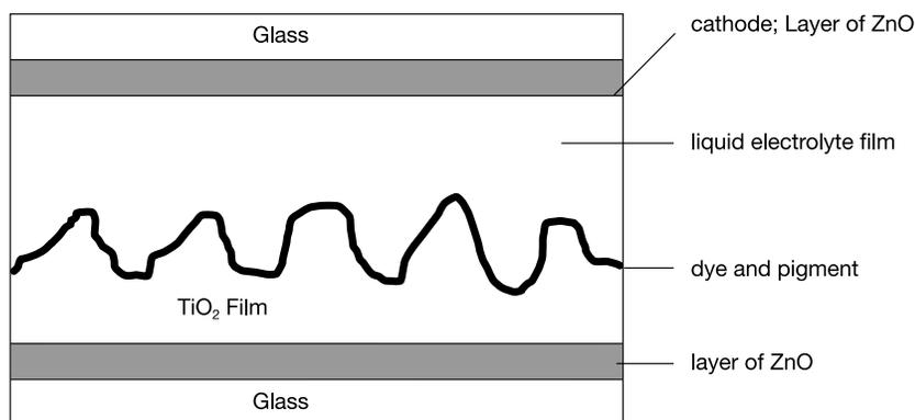
**Figure 4.** Construction of a Graetzel cell (reproduced from Volker and Hoffmann (1996)).
