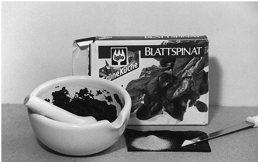
**Figure 2.** Materials for the Graetzel cell: spinach, titanium dioxide (e.g., toothpaste), a knife tip of calcium carbonate.
